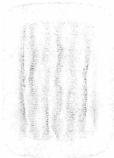
Figure 5.9 High twist weft inserted every 4 th pick. Sample 12
