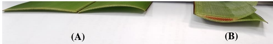
Figure 3.3. Cross-section of the cut ends of the flax top (FT) and bottom (FB) sections. (A) cross-section of the cut end of the flax top section, (B) cross-section of the end point of the flax top section and beginning of the flax bottom section.
