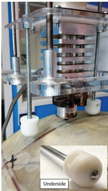
Figure 5-5: Guides resting on platform to keep the nozzle height constant.
