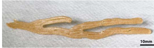
Figure 5-8: Extrusion quality of 4 RPM motor
