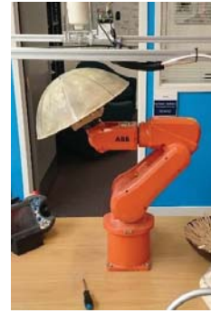
Figure 3-3: Robot with platform attached
