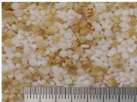
Fig. 1 Blended pellets of biopolyesters containing approx. 5 wt.% of Phormium tenax fibre. Smaller units on the scale = 0.5 mm.
