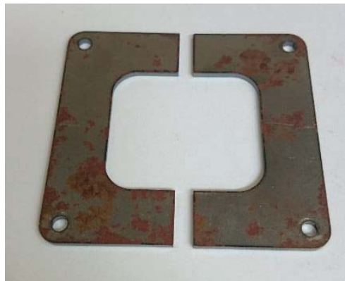
Figure 3-23: 2 mm laser cut steel plates
