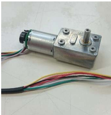
Figure 3-22: Worm gear driven 4RPM motor
