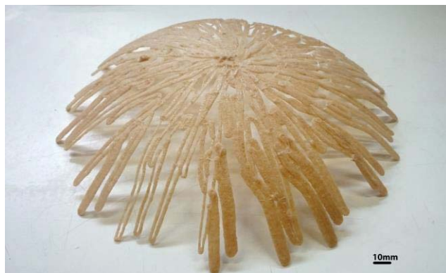
Figure 5-2: Flow inconsistency of extrusion
