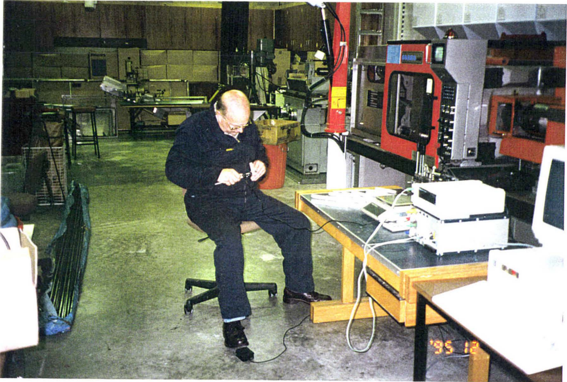
Figure 3.10 Measuring the product dimensions using the pedal switch
