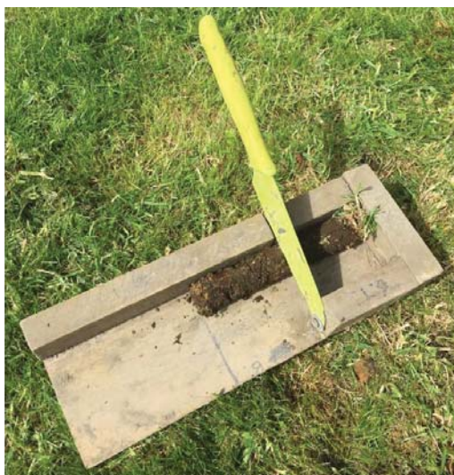
Figure 3.6. Improvised soil core sectioning device used to separate 0-75 mm and 75-150 mm sub-samples (photograph courtesy of the author).
