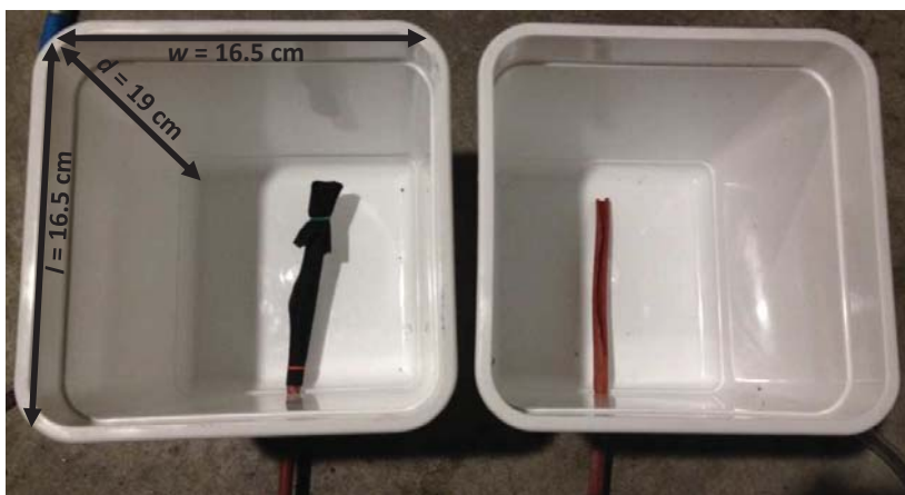
Figure 7.1. Design of pots (left, completed; right, partially complete showing the slit in the internal drainage tube) used for generating cyclical 3-day flooded, 11-day drained soil conditions (photograph courtesy of the author).
