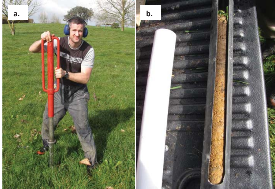
Figure 3.7.a) Device used to collect intact soil cores from the field, and b) Example of intact soil core (still inside the corer) and adjacent PVC pipe used to transport the intact cores (photographs courtesy of Michael Hedley).
