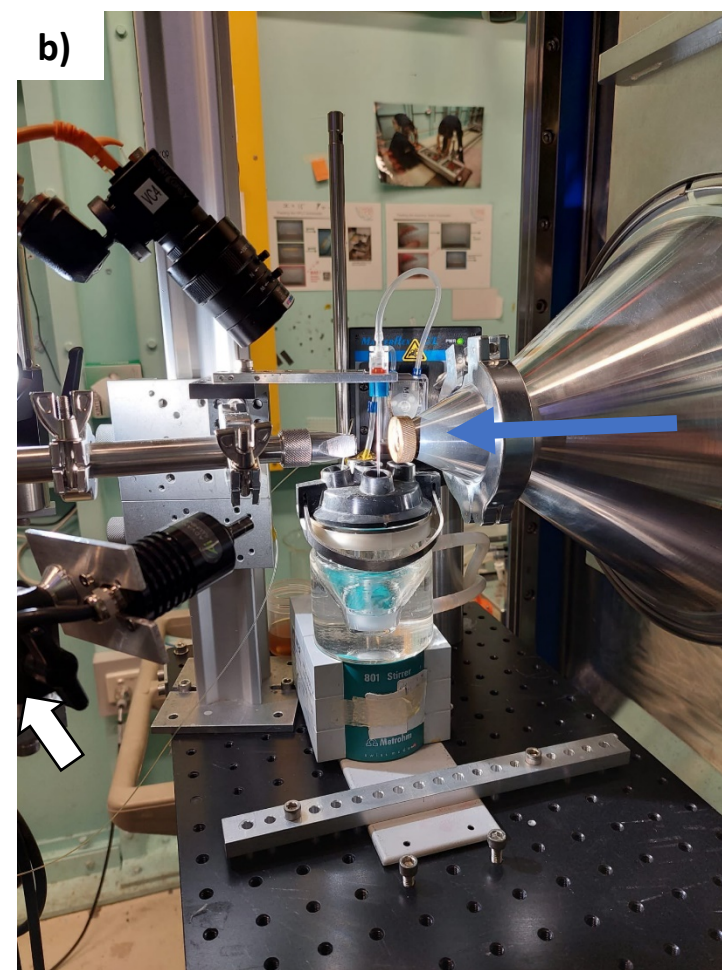
Appendix 7.2. Front (a) and back (a) of detergent-induced vesicle \rightarrow micelle transition SR-SAXS experiment set-up. Thin tubing (white arrow) remotely injects bile from a syringe driver (not pictured). Blue arrow indicates the direction of the x-ray beam. Glass vessel holds and stirs the phospholipid vesicles. Solution is stirred in the vessel and aspirated through the capillary via peristaltic pump. Clamp holds the capillary and stand holds the stirrer plate and vessel in place.
