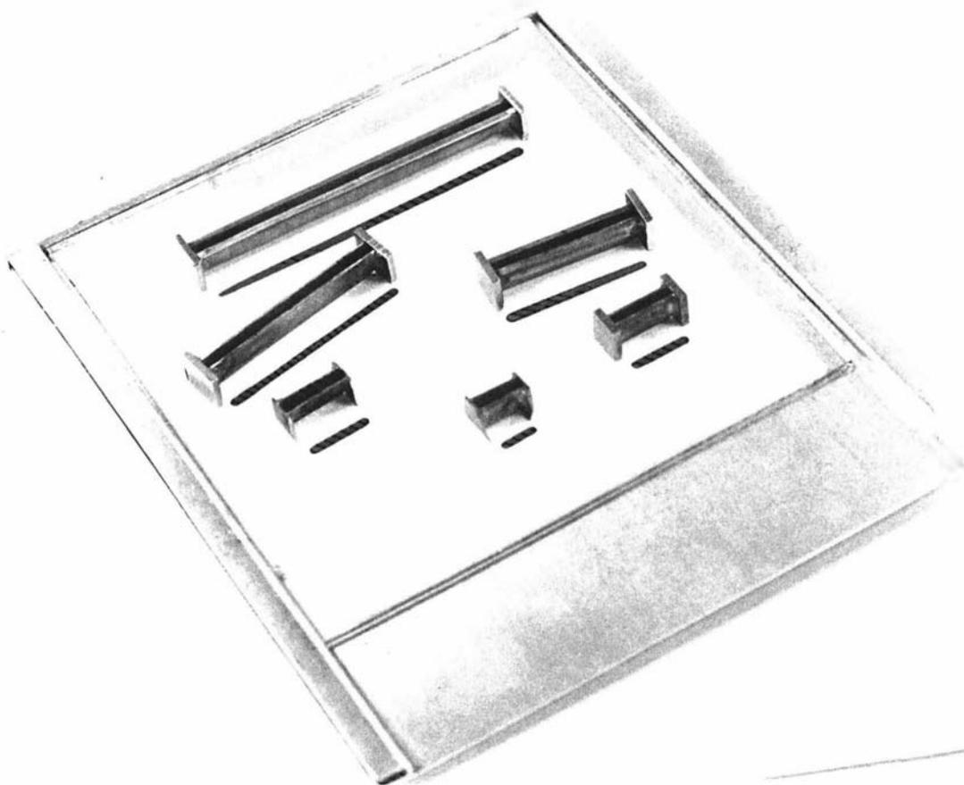
Fig. 1.3. Some of the sample streakers in routine use in this laboratory arranged on a  $(20 \text{ cm})^2$  layer ( $250 \mu$ ) of Silica Gel H. The thin streaks produced by the devices are displayed in front of each one.
