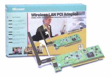
Figure 7.2 Micronet SP906B PCI wireless interface with the ADM8211 chipset
