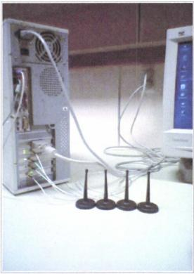
Figure 7.4 Different views of the four wireless interfaces installed in the computer showing also the antennas used. The top three interfaces are the ADM8211 chipset interfaces while the bottom interface is the RTL8180L chipset interface
