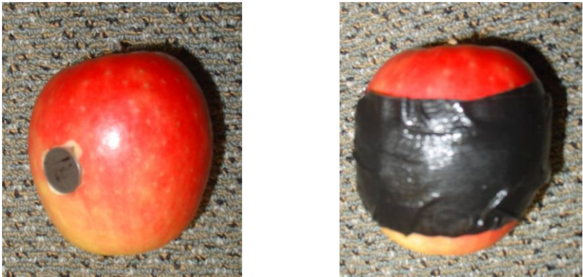
Figure 6.2, Placement of I-button temperature sensor for purpose of monitoring apple temperature during fruit grading and packaging.
