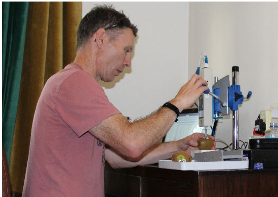
Figure 3.2: GY-4 digital fruit penetrometer used for kiwifruit firmness assessment.
