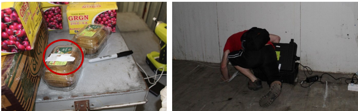
Figure 3.1: Data loggers attached on kiwifruit punnets for monitoring storage conditions at street vendors stores (left). Setting up the ethylene monitoring equipment in one of the importers cool stores in India (right).
