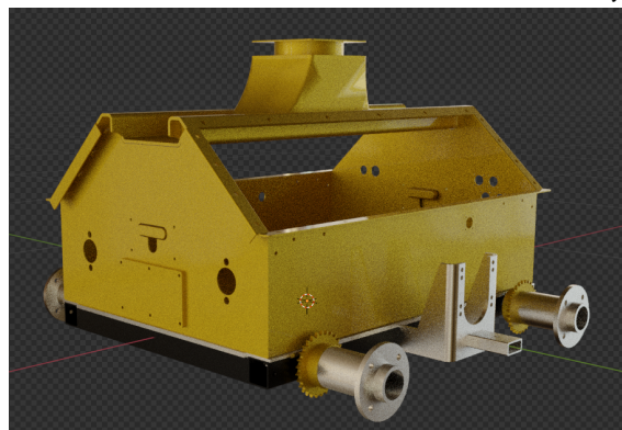
(c) Digital Twin chassis with materials added for export to Collada .dae format.
