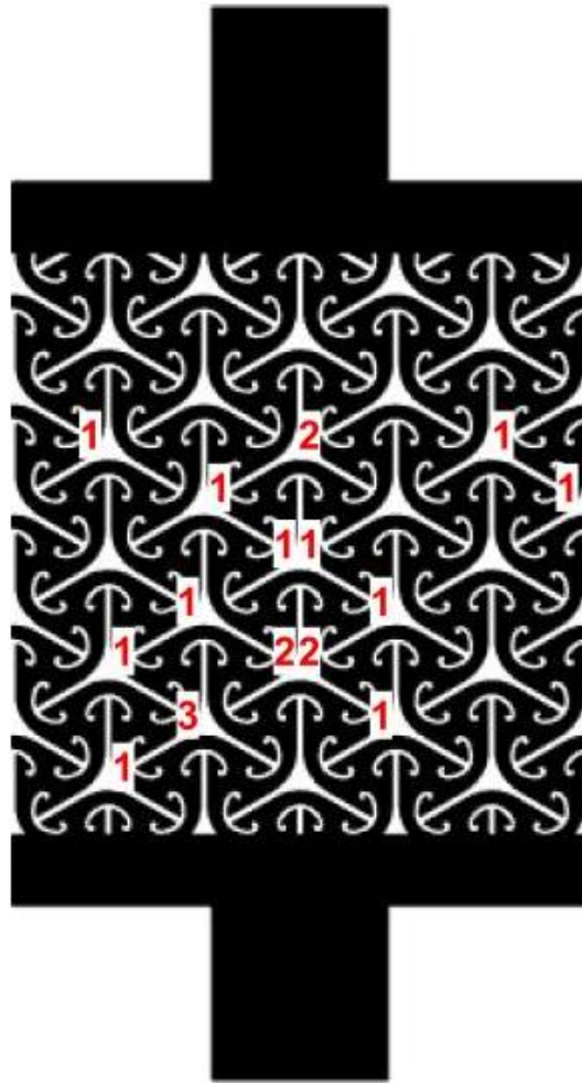
Figure 17 - Hinge failure locations of 3x5 grid across twenty test replicates
