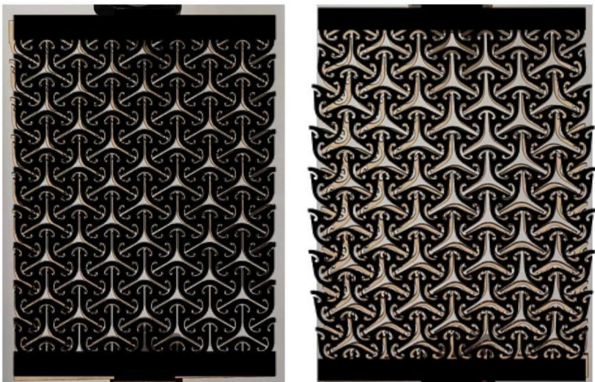
Figure 27 - Overlay of Comsol model (black overlay) and experimental images (background) for 4x8 grids at 0 mm displacement (left), and 3 mm displacement (right).
