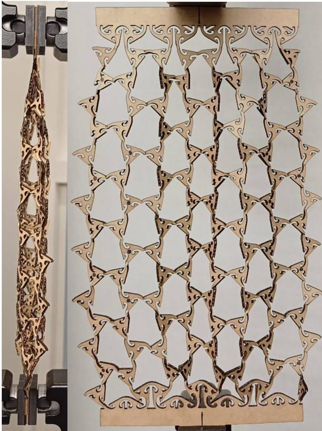
Figure 20 - Out-of-plane behaviour of the auxetic under tension. Side view (Left) and Front view (Right)
