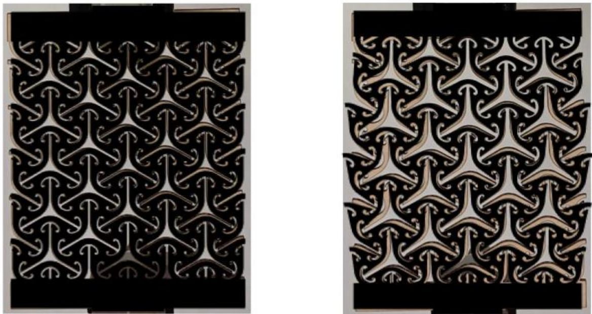
Figure 26 - Overlay of Comsol model (black overlay) and experimental images (background) for 3x5 grids at 0 mm displacement (left), and 2 mm displacement (right).
