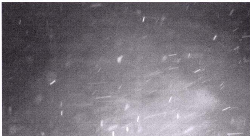
Figure 4.16: Example frame for water at 0.5 bar atomization pressure and 1.8 \text{ kg h}^{-1} .
