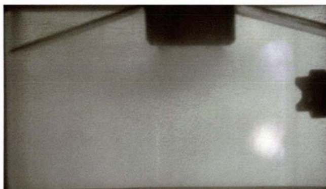
Figure 7.15: Fines curtain shape with 1.5 bar atomiser air (D2b).
