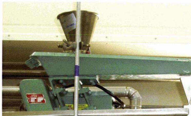
Figure 5.10: Hopper and vibrating chute.
