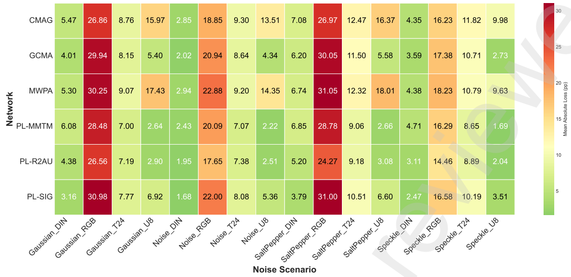
Figure 17: Scenario-level noise sensitivity heatmap (modality \times noise type). Cell intensity represents mean absolute loss (pp) across networks, lighting conditions, and intensity levels. Gaussian noise on RGB constitutes the worst-case scenario (28.84 pp, 35.0% relative degradation). RGB-targeted corruption dominates across all noise types, while DIN and UV corruptions induce substantially lower degradation for most architectures.
