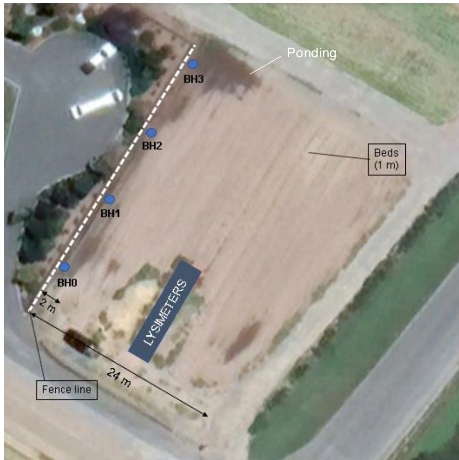
Figure 3.9. Location of piezometers in the field at the Green vegetables site (BH1 for piezometers 1 (1 m depth), BH2 for piezometer 2 (5 m depth) and BH3 for piezometer 3 (1 m depth)).
