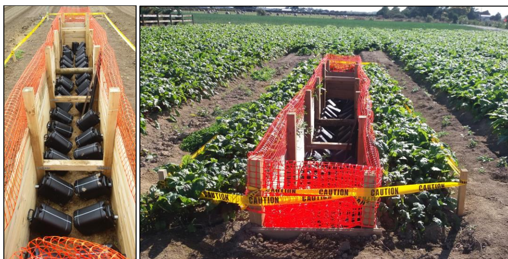
Figure 3.6. Installation of lysimeters at the Green vegetables site.
