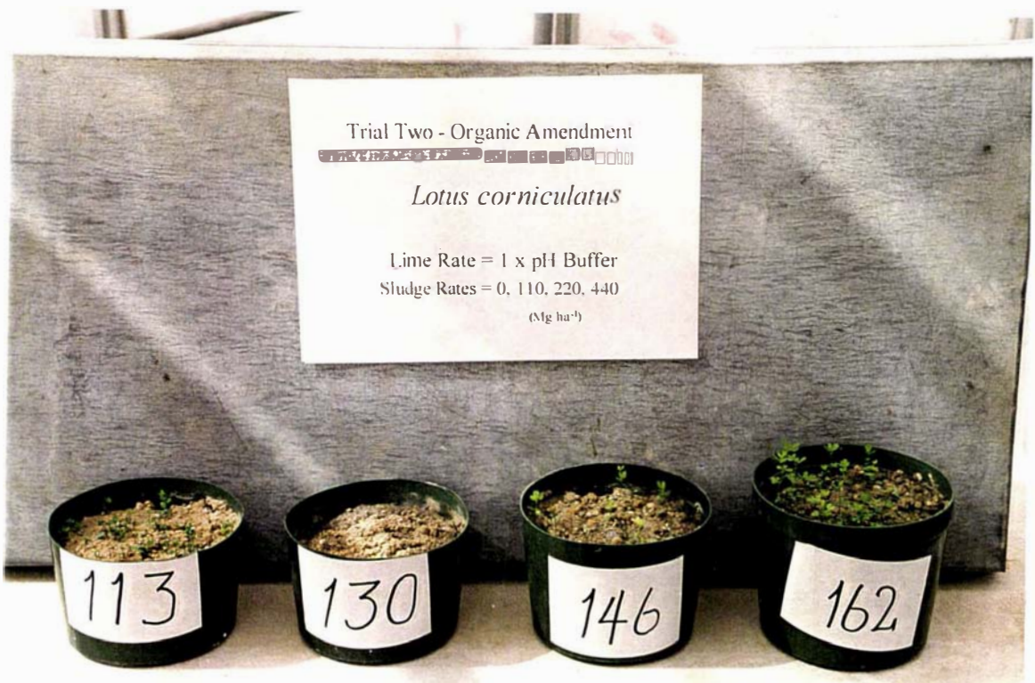
Plate 7.9 This photograph was taken 4 weeks after sowing and compares the growth of Lotus corniculatus on tailings amended with 4 rates of sludge (nil, 110, 220 & 440 Mg/ha; left to right) and 4 rates of lime (16.5, 10.1, 8.5 & 5.1 Mg CaCO 3 /ha; left to right).
