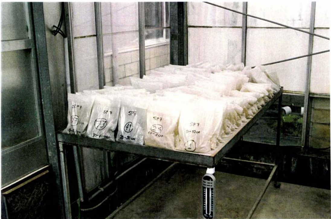
Plate 6.1 Lime Incubation Experiment January 1995. Polyethylene bags containing lime amended tailings
