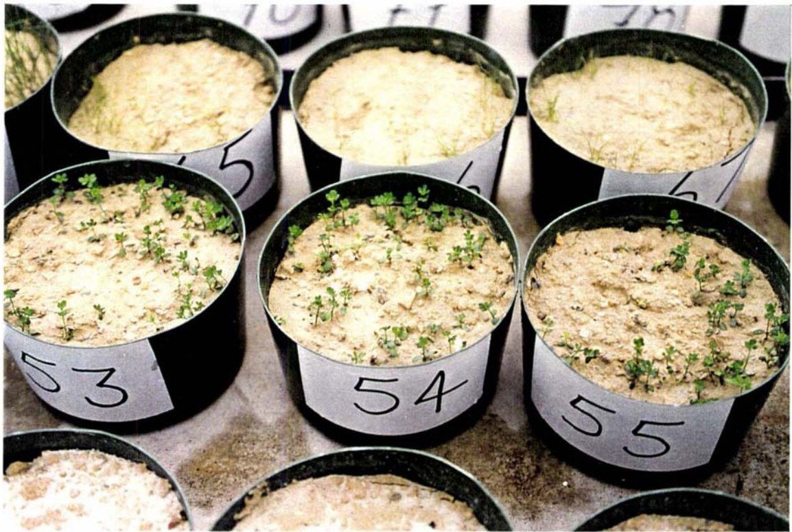
Plate 7.4 The Lotus corniculatus seen growing in this photograph (pots 53-55) are about 4 weeks old and are clearly performing poorly. Grown in tailings limed at a rate of 16.5 Mg/ha the plants showed signs of chlorosis and a generally yellow stunted appearance, symptoms consistent with N deficiency.
