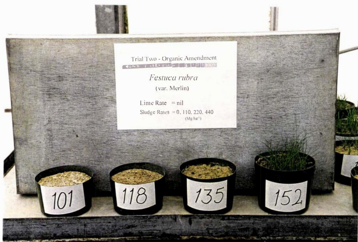
Plate 7.7 This photograph taken 4 weeks after sowing compares the growth of F. rubra (Merlin) grown on tailings amended with 4 different rates of sludge; nil, 110, 220 and 440 Mg/ha. Sludge rate increases from left to right.
