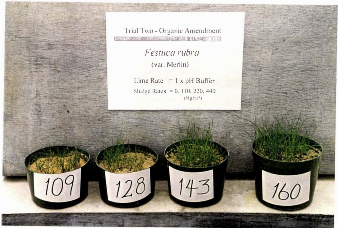
Plate 7.8 This photograph was taken 4 weeks after sowing and compares the growth of Festuca rubra (Merlin) on tailings amended with 4 rates of sludge (nil, 110, 220 & 440 Mg/ha; left to right) and 4 rates of lime (16.5, 10.1, 8.5 & 5.1 Mg CaCO 3 /ha; left to right).
