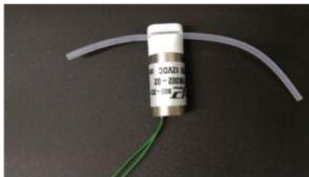
FIGURE 4.5: Schematic of the pinch type valve
