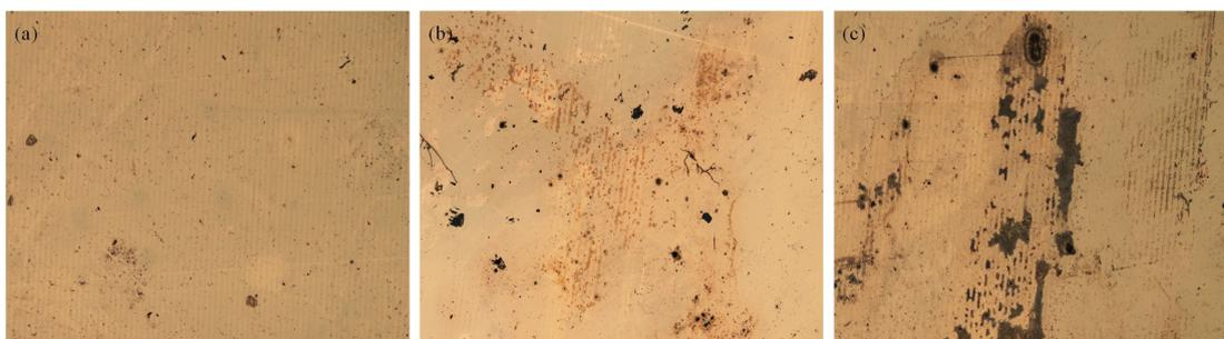
FIGURE 5.19: Optical micro-graph of GSH patterns (a) Before arsenic exposure, (b) After As(III) (20  $\mu\text{g/L}$ ) exposure, (c) After As(III) (50 $\mu\text{g/L}$ ) exposure.
