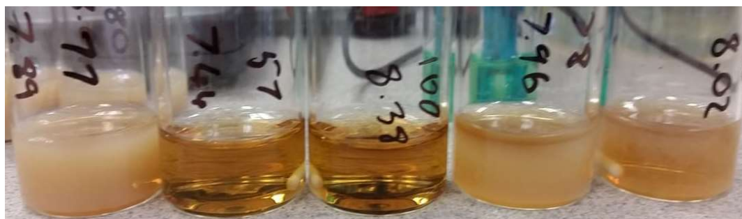
Figure 25 - Picture taken of solutions made during ns241. The right number written on the vial is the amount of KOH (6.011 M) added in \mu\text{L} and the left number is the resulting pH. These solutions were made in order of left to right. The picture was taken ~10 minutes after the last vial was made. The contrast in the cloudiness of the solutions shows that solutions closer to pH 8.00 form the K-TA coordination polymer much faster and that a difference of 0.5 in pH has a significant effect on K-TA formation.
