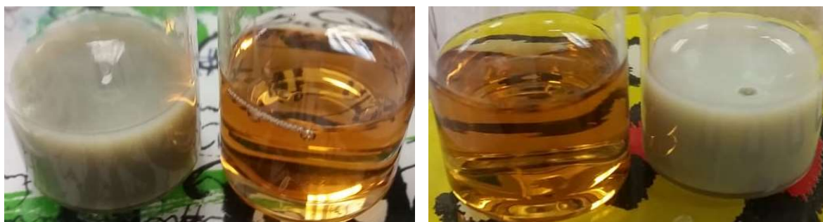
Figure 28 - Pictures showing K-TA solutions (inner vials) compared to the ZIF-8 solutions to which the K-TA was added (outer vials). The pictures were taken ~15 minutes after the K-TA solution was added to the ZIF-8 solutions.
