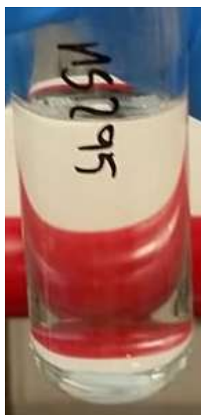
Figure S114 - Image showing the clarity of the reaction mixture. By eye, no catalyst remains in the solution.
