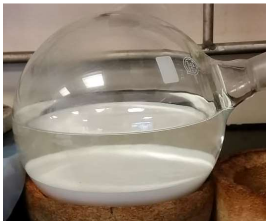
Figure 22 - Image taken of vessel left on angle during 24 hours that ZIF-8 is left to incubate at room temperature. The white solid ZIF-8 has settled at the bottom of the vessel and the remaining solution is ready to pour off.
