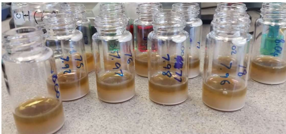
Figure S14 - Picture taken of the solutions shown in Figure 26 and Figure 27 in the main text after leaving them overnight. This shows that K-TA solutions form the green by-product (the dark green top layer of solution) eventually, regardless of pH, as the pH just affects the rate of formation. Note that the desired K-TA that has formed has sunk to the bottom to form a thin layer of solid.
