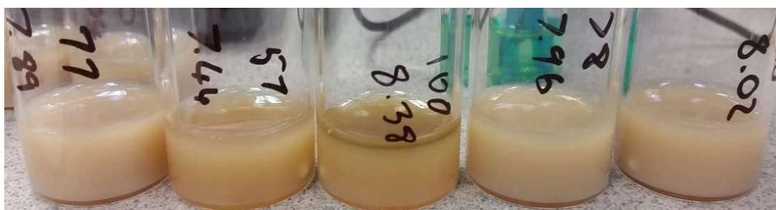
Figure 26 - Picture taken of solutions made during ns241. This picture was taken ~1 hour after the picture taken in Figure 25. This shows that a pH varying 0.5 from 8.0 (i.e. 7.5 and 8.0) will still form K-TA, albeit much slower than it would at a pH of 8.0. The centre vial (at a pH of 8.38) also shows signs of a green phase forming on top of the solution. This green phase is an undesired by-product that forms faster at higher pH.
