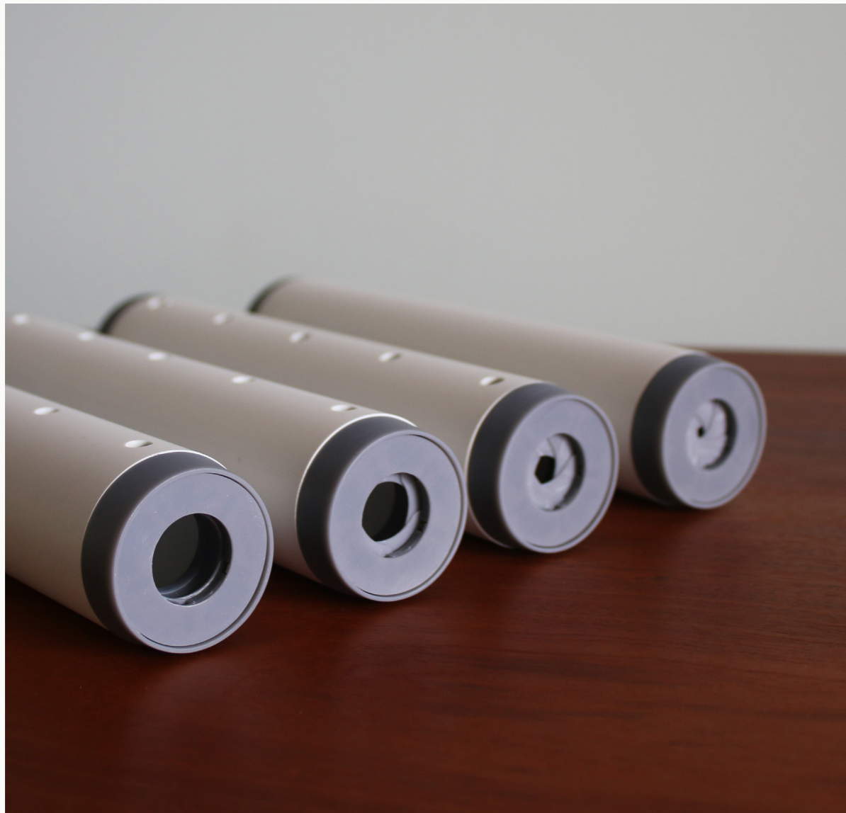
Fig. 55. Close up of the tuning dial showing the full range of aperture diameters
