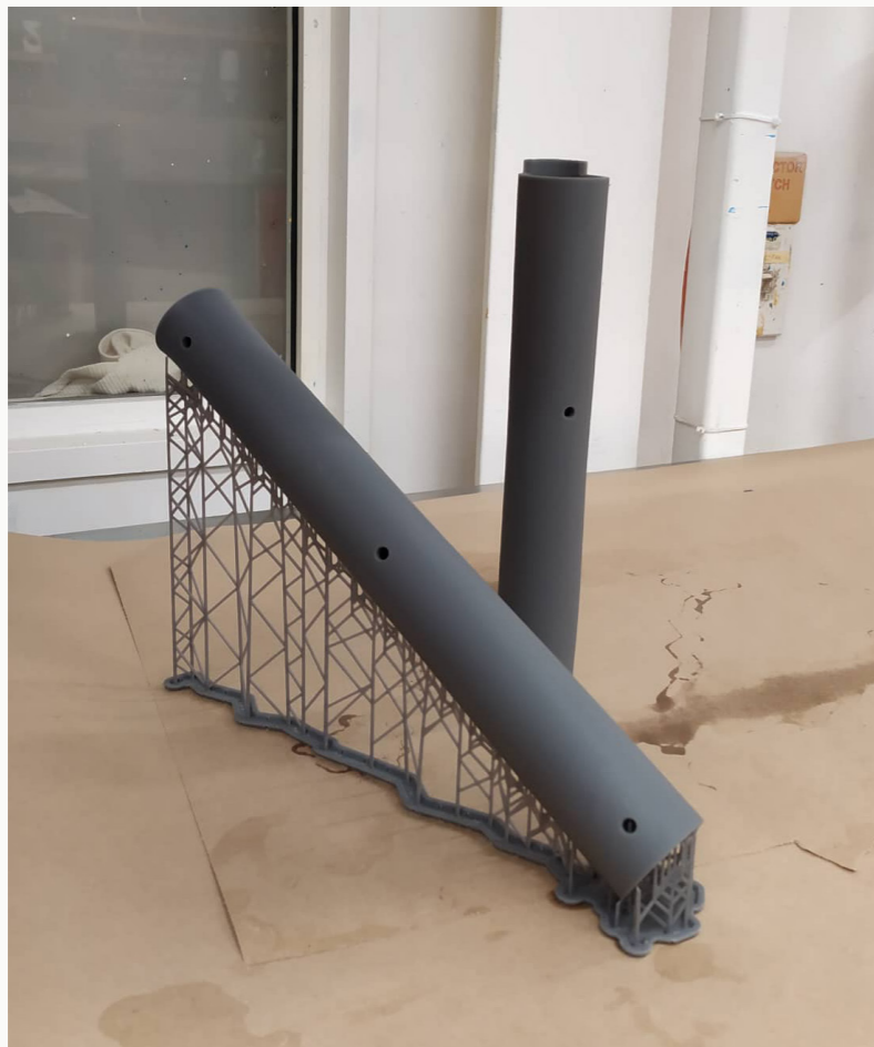
Fig. 31. Photograph of SLA printed fangufangu artefact FE012471. Due to its size, this was printed in two parts
