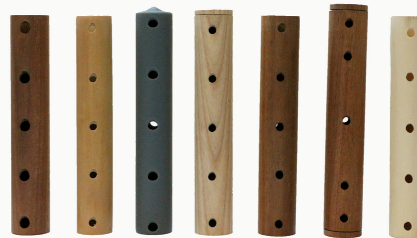
Fig. 18. Photograph of 7 fangufangu made from different variations of bamboo, timber and plastic. This focussed on understanding implications of sound across different materials and finger hole variations for same or similar dimensions.
