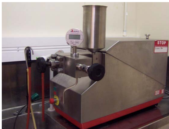
Figure 3.2-1: Lab scale two-stage valve homogenizer (APV 2000, Silkeborg, Denmark).
