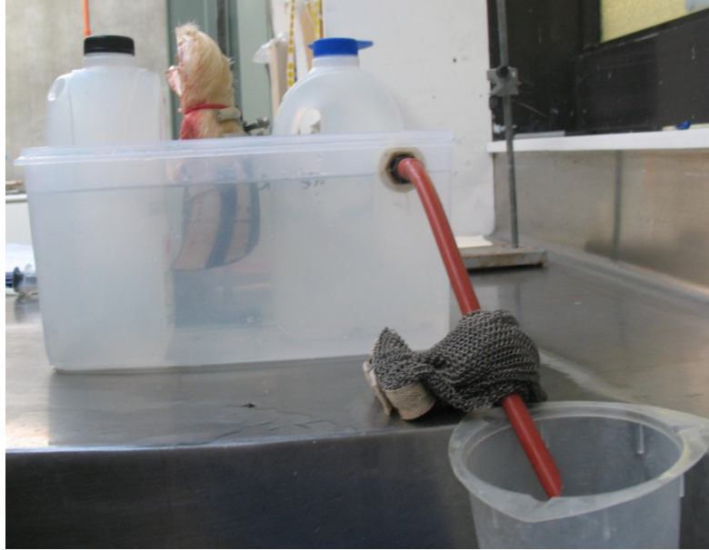
Figure 2.1b: water displacement equipment after Scott et al. (1999). Water displaced by the claw overflows to collection vessel via rubber tubing.
