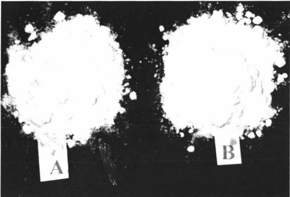
Fig. 5.1 The appearance of the powdered fats after standing for five minutes at ambient temperature; A = Unmodified AMF; B = SBF42 (Hard Fraction).
