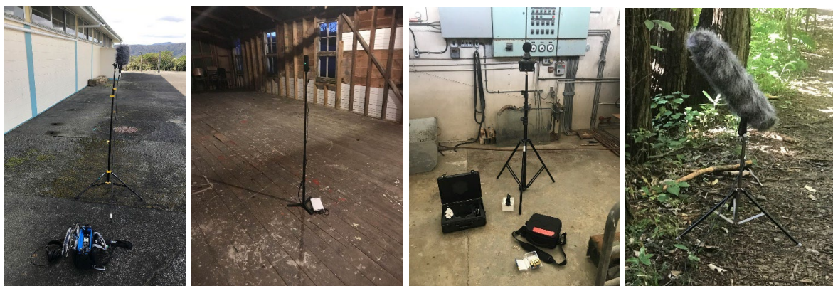
(fig. 96) Doidge, M. (2019). Left, Ambisonic mic and Zoom F8 recorder. Middle Left, Insta Onex 360° 6 k monoscopic camera + 30000 mAh battery. Middle Right, Kandao 8k stereoscopic camera + Zoom H3 ambisonic recorder. Right, Sennheiser T - power shotgun mic. Courtesy the artist.
