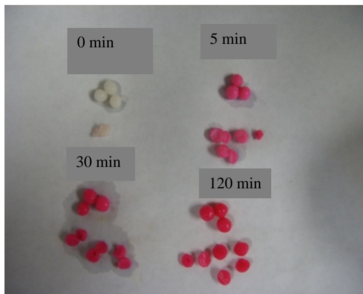
Figure A.6 Colour changing inside the beads after being put in methyl red-stained SGF: the colour inside the beads varied from colourless to red.
