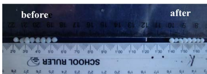
Figure 3.1 Alginate- \text{CaCl}_2 beads before and after incubation in SGF.
