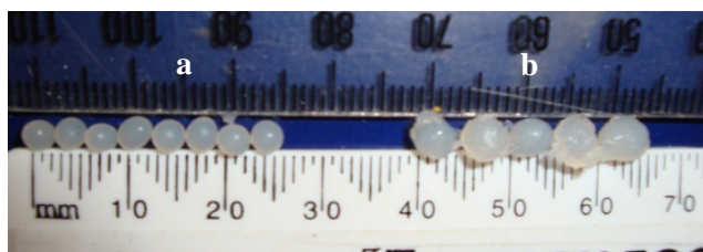
Figure 3.4 Alginde- \text{Ca}^{2+} -chitosan (chitosan dissolved in calcium chloride first) beads before and after coating with 1% alginde. (a) alginde-( \text{CaCl}_2 -chitosan) beads; (b) (alginde-( \text{CaCl}_2 -chitosan))-alginde beads
