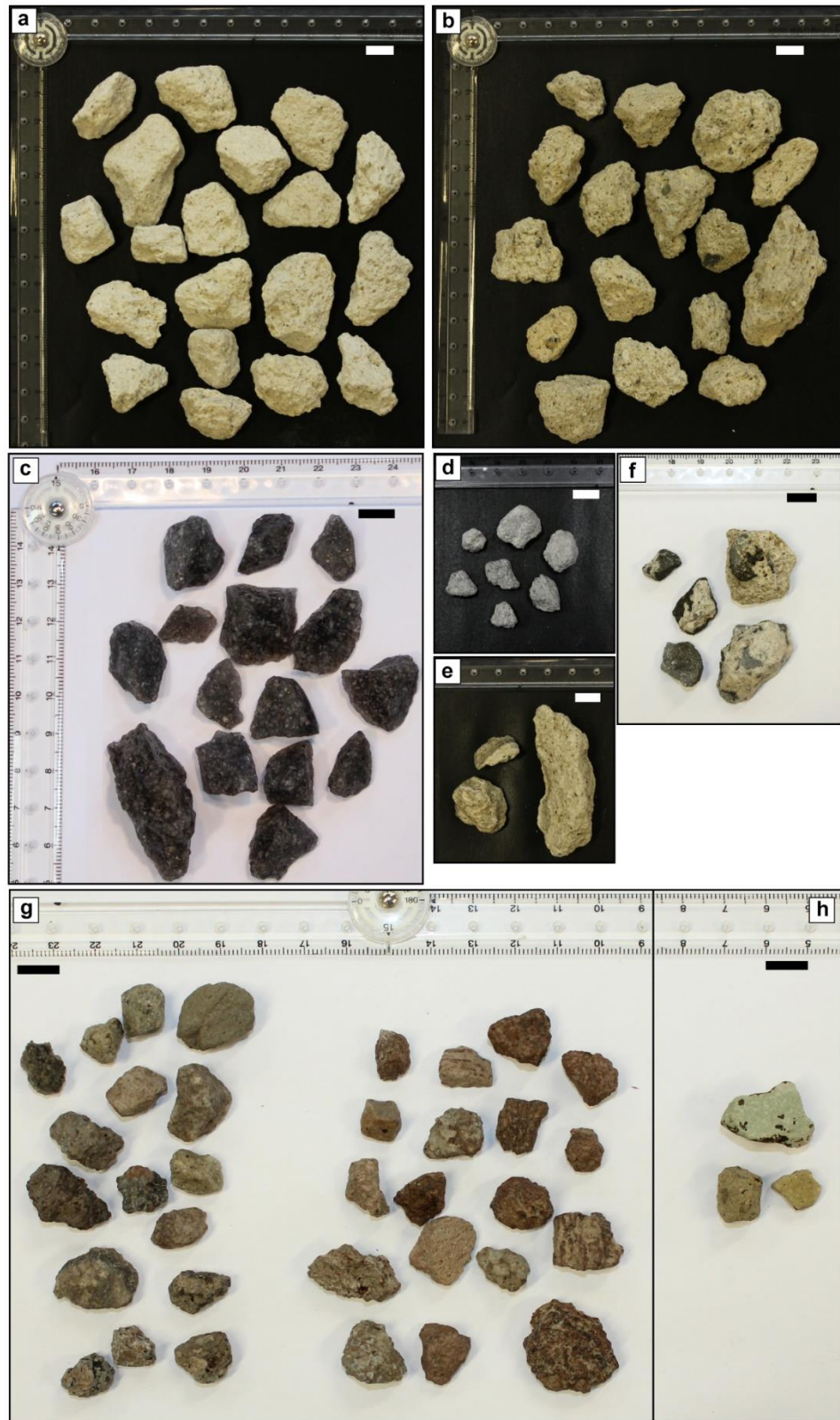
Figure 3.14 – Representative clasts photographs of juvenile ( a to f ) and lithic ( g and h ) materials of the Kaharua deposit: ( a ) white pumice; ( b ) grey pumice; ( c ) obsidian; ( d ) dense juvenile; ( e ) banded pumice; ( f ) basaltic material as free clasts and coated with pumice; ( g ) lava fragments with variable degree of oxidation; ( h ) hydrothermally altered clasts. White and black scale bars are 1 cm long in each picture.
