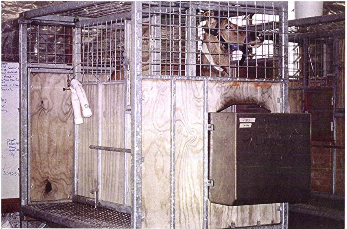
Plate 3.1 Hind housed in a metabolism cage and wearing methane-collecting apparatus, with the yoke attached near the rear of the sliding door of cage.
