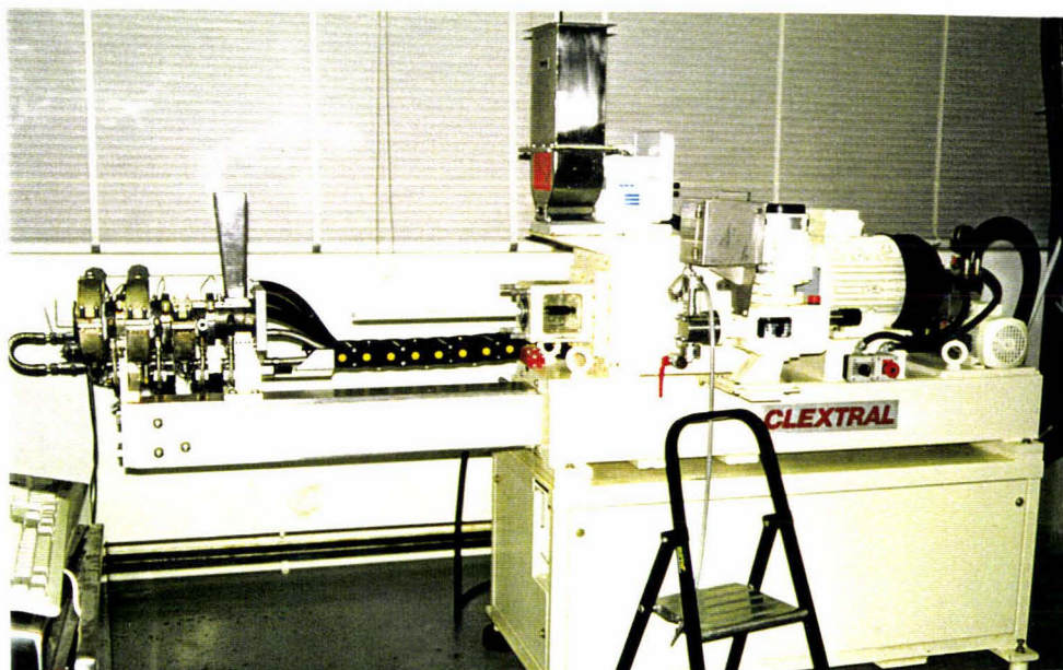
Figure 4.1 Twin screw extruder (Clextral BC-21, France)
