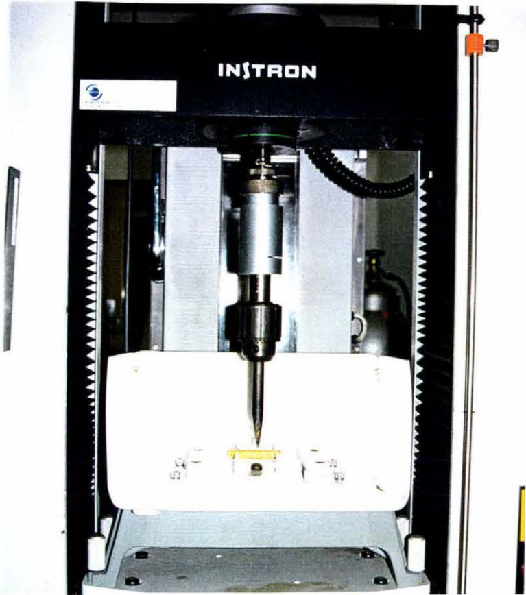
Figure 4.5 Chisel probe for testing extrudate samples
