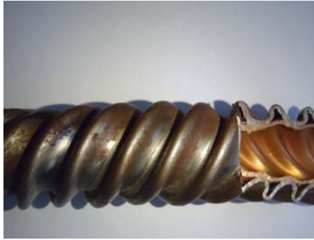
Figure 4.6: Possible twisted tube if big difference in size between the 1 st and 2 nd tubes
