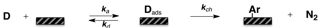
Scheme 5.2. Two-stage model representing the mechanism for grafting of an aryldiazonium to a surface.
