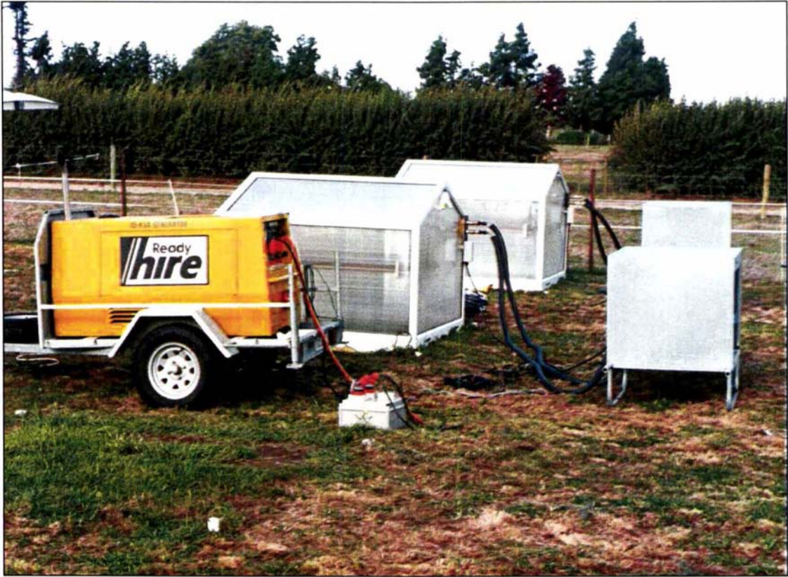
Plate 4-2 Computer-regulated transparent-polycarbonate chambers, with generator and refrigeration units. Applying heat treatment at the Bay of Plenty site, February 1998.
