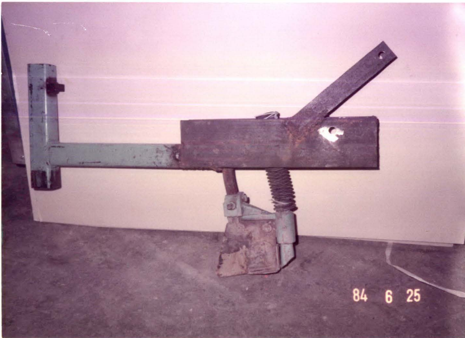
Figure 4.2.2d 1000 winged opener assembly. Top. With depth control wheels. Bottom. Without depth control wheels.
