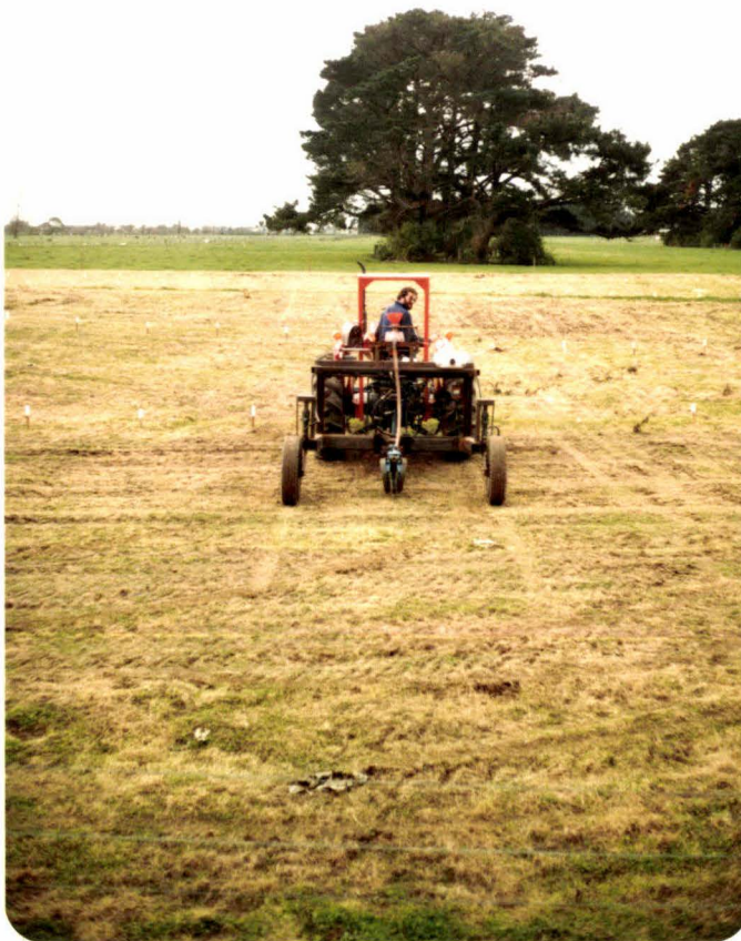
Figure 4.2.2e Test rig with a single opener and cone seeder assembly.
