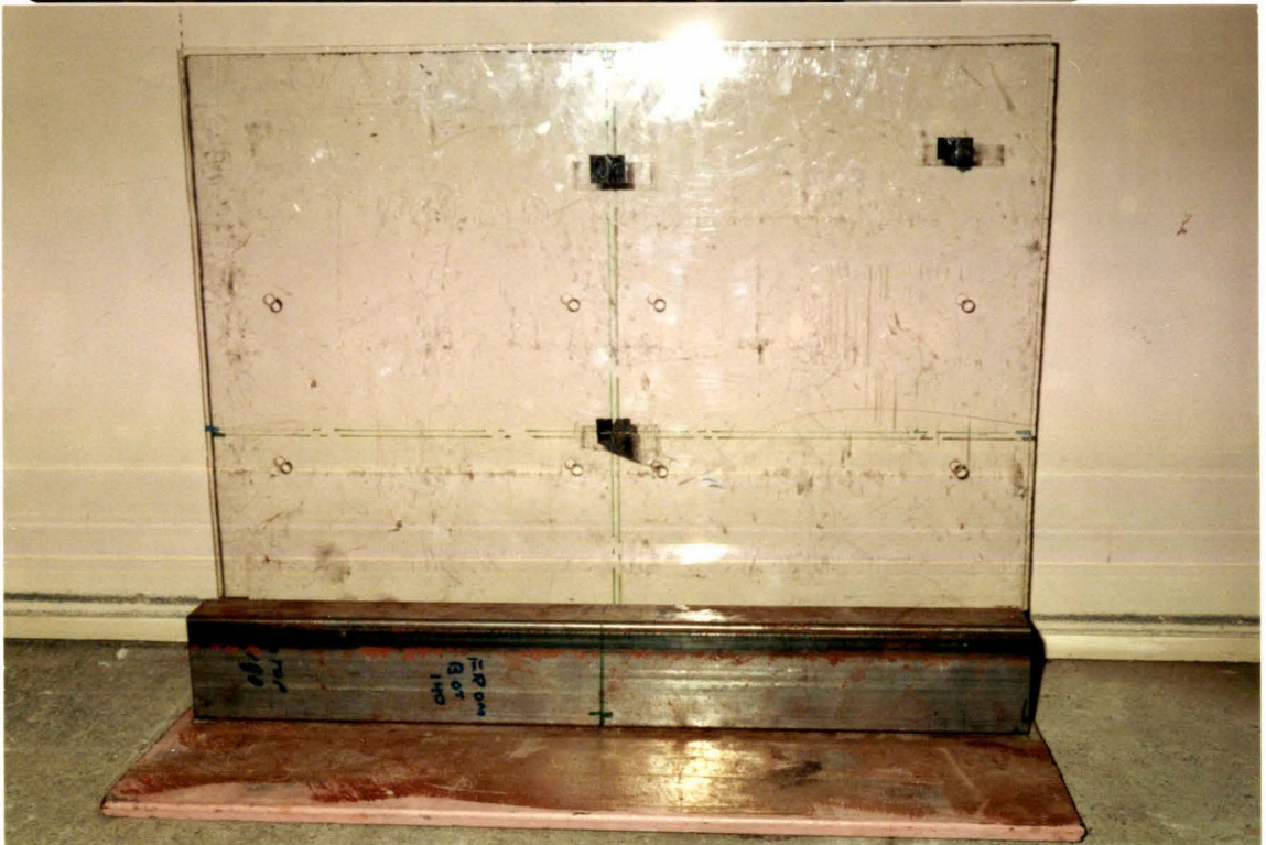
Figure 3.9.3. Soil block positioning jig.
