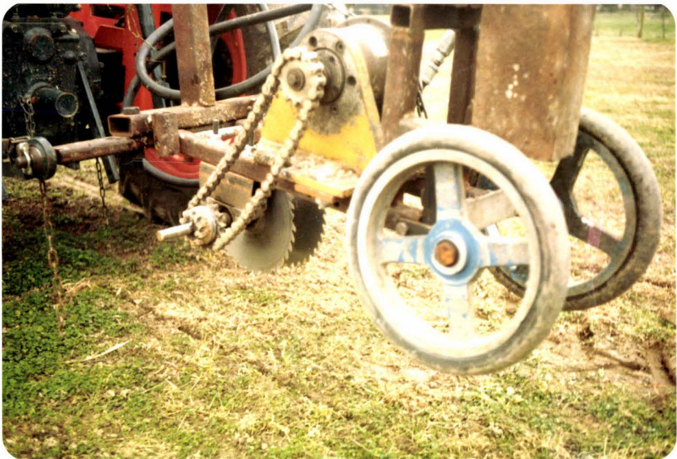
Figure 3.9.1. Soil block cutting machine.
