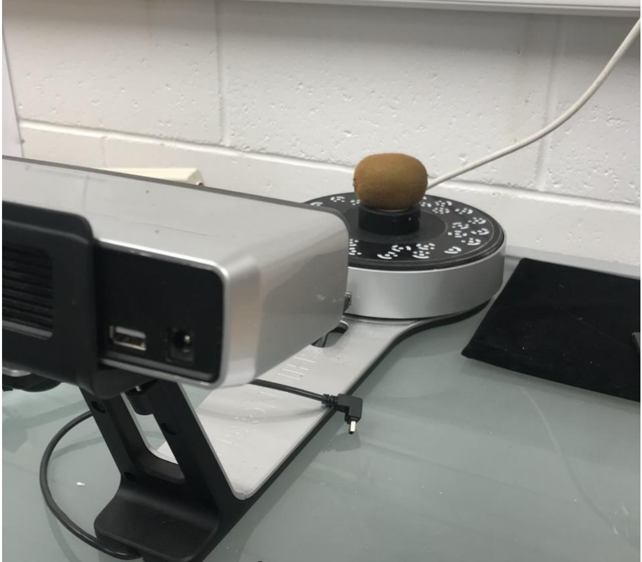
Figure 14. Kiwifruit being scanned by the SHINING 3D using a black plastic base (one of the bases trialled for experiments).
