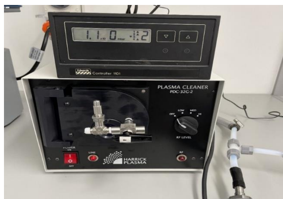
Figure 2.2.3. 1 Plasma cleaner showing the needle valve, plasma cleaner and pressure gauge.
