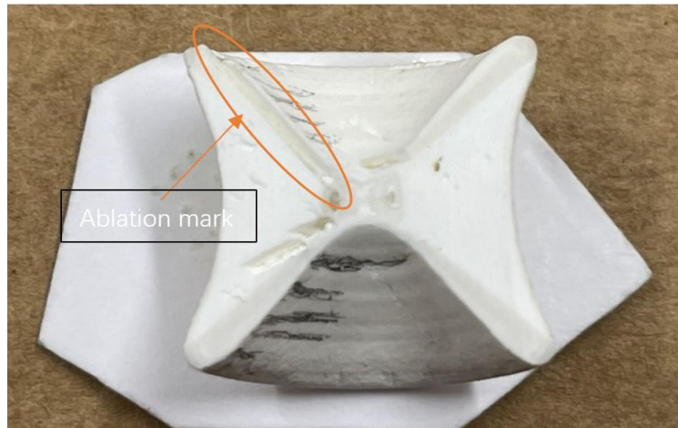
Figure 3.4.3.2. 2 The ablation mark on the surface of shark vertebra half.
