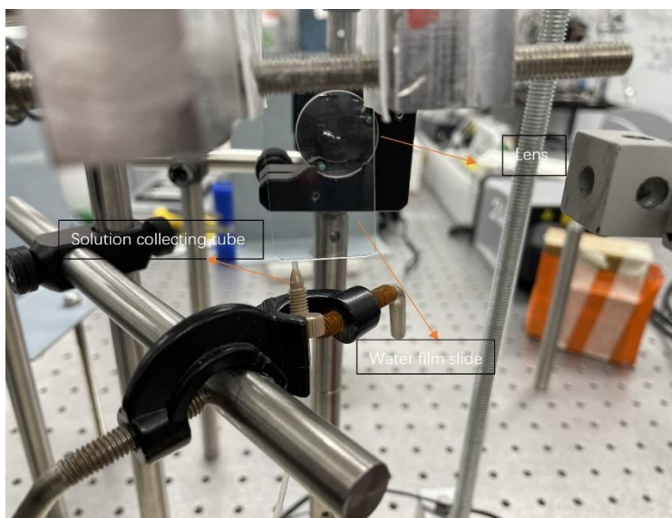
Figure 2.3. 4 The position of the lens and the FC glass slide setup.
