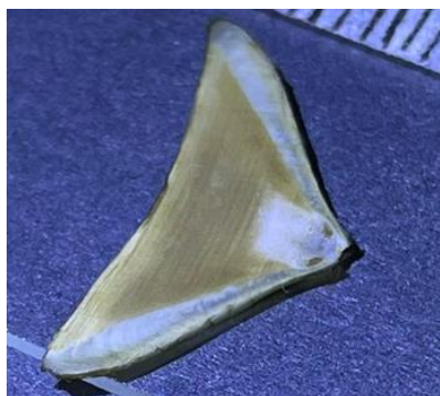
Figure 3.4.6.3. 2 Sample SWS5-D1, part 1. Indirect light: Both growth marks and saw marks were shown.
