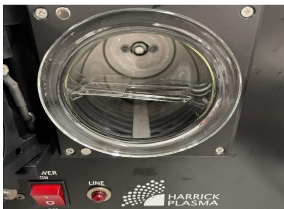
Figure 2.2.3. 2 The chamber of the plasma cleaner with slides in situ.
