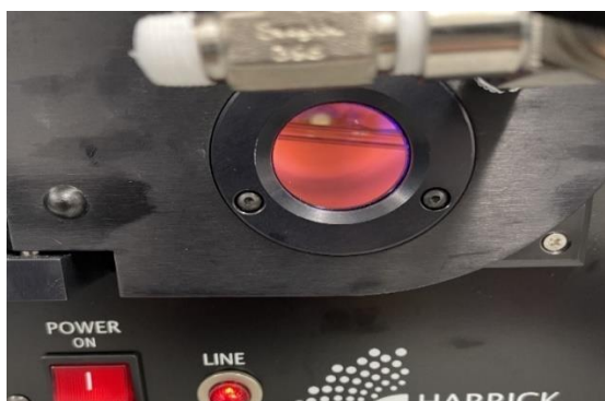
Figure 2.2.3. 3 The cleaner is on and under the high RF mode the glow from the plasma is clearly visible.
