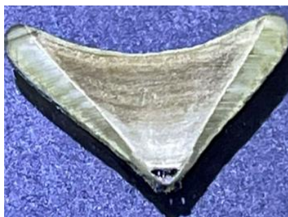
Figure 3.4.6.3. 2 Sample SWS5-D1, part 1. Indirect light: Both growth marks and saw marks were shown.
