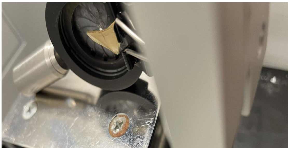
Figure 3.4.4.2. 2 The position of the vertebra section behind the iris.
