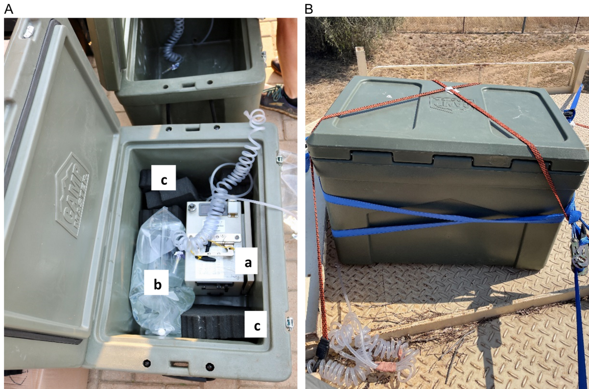
FIGURE 6 | (A and B) Infusion pump (a) along with one drip bag (b) and pieces of foam (c) for protection and positioning of the drip bags in the 60-L cooler box (A) and the cooler box strapped down on top of the rhinoceros crate (B).
