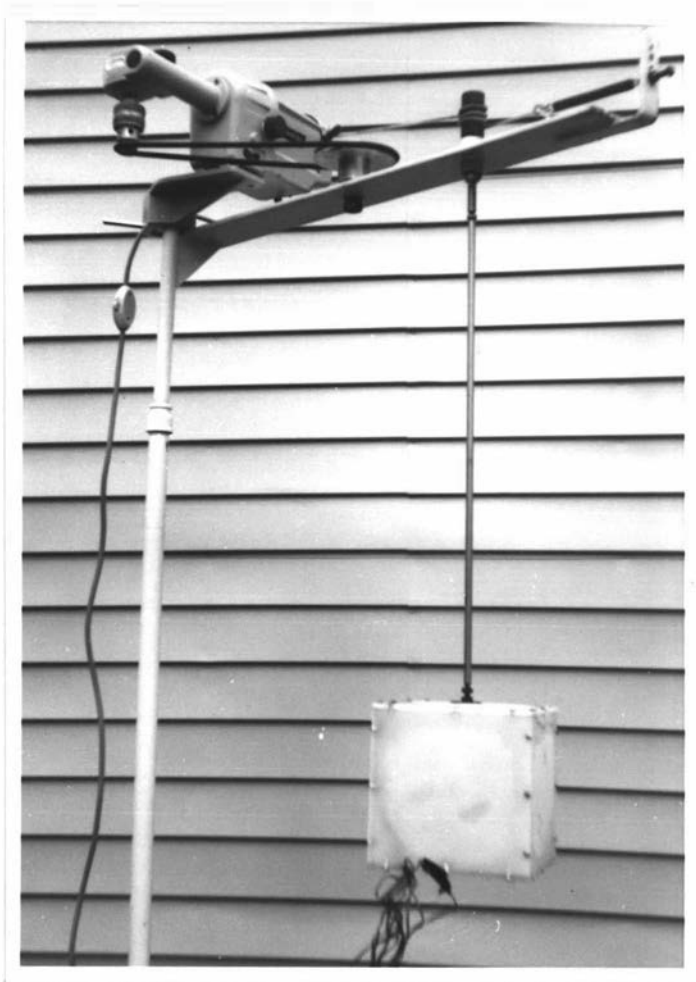
Figure 4.13 Typical polypropylene containers used in the experimental investigation into freezing of rectangular bricks.
