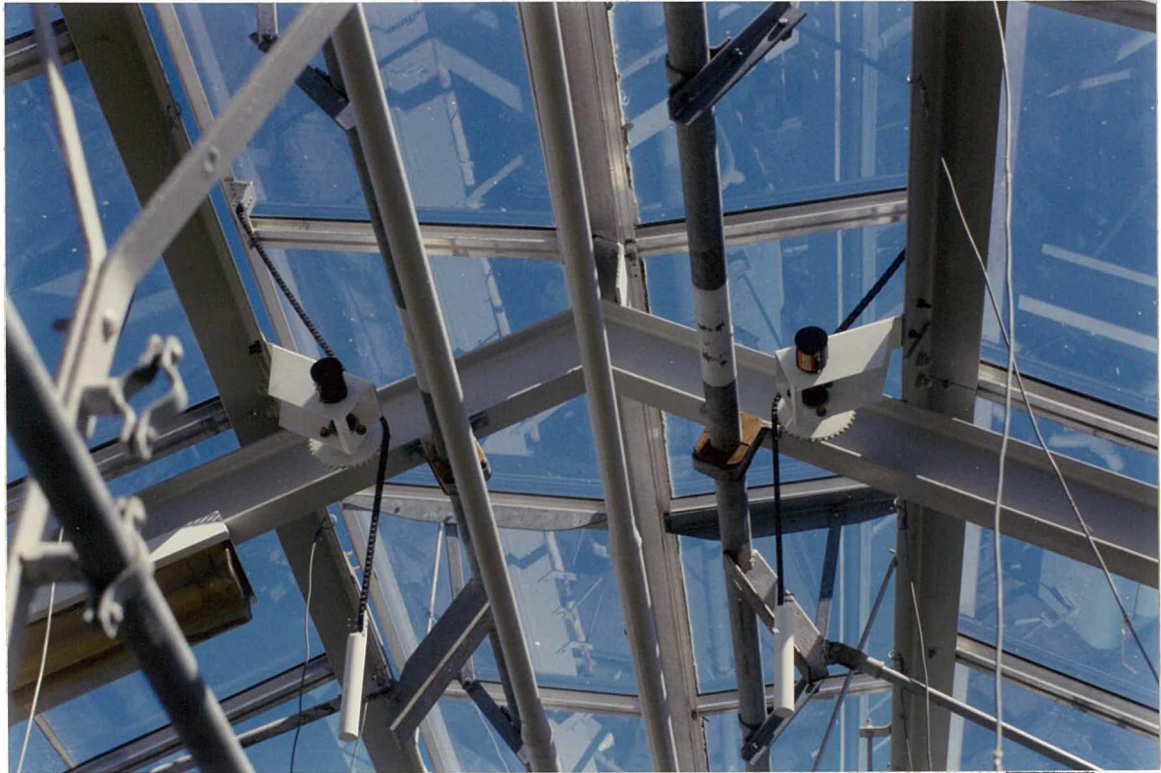
Plate V. Window opening Measurement System.
