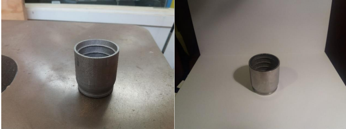
Figure 4.24. Item SMSNS-16: Before & After Polishing
