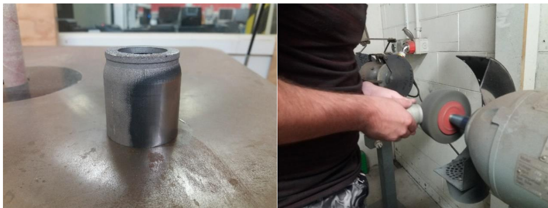
Figure 4.23. Item SMSNS-16: Polishing Process
