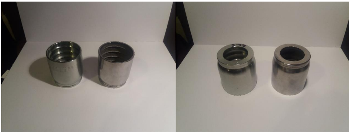
Figure 4.25. Item SMSNS-16: The Traditional Manufactured (left) and the 3D Printed (right) Items
