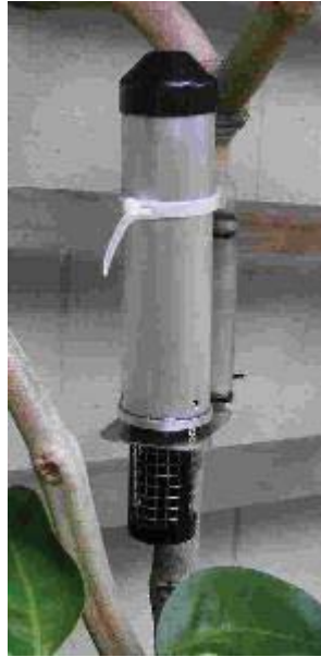
Figure A6.3. Mounting the recorder on a tree.
