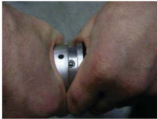
Figure A6.1. Removing the cover of the recorder.
