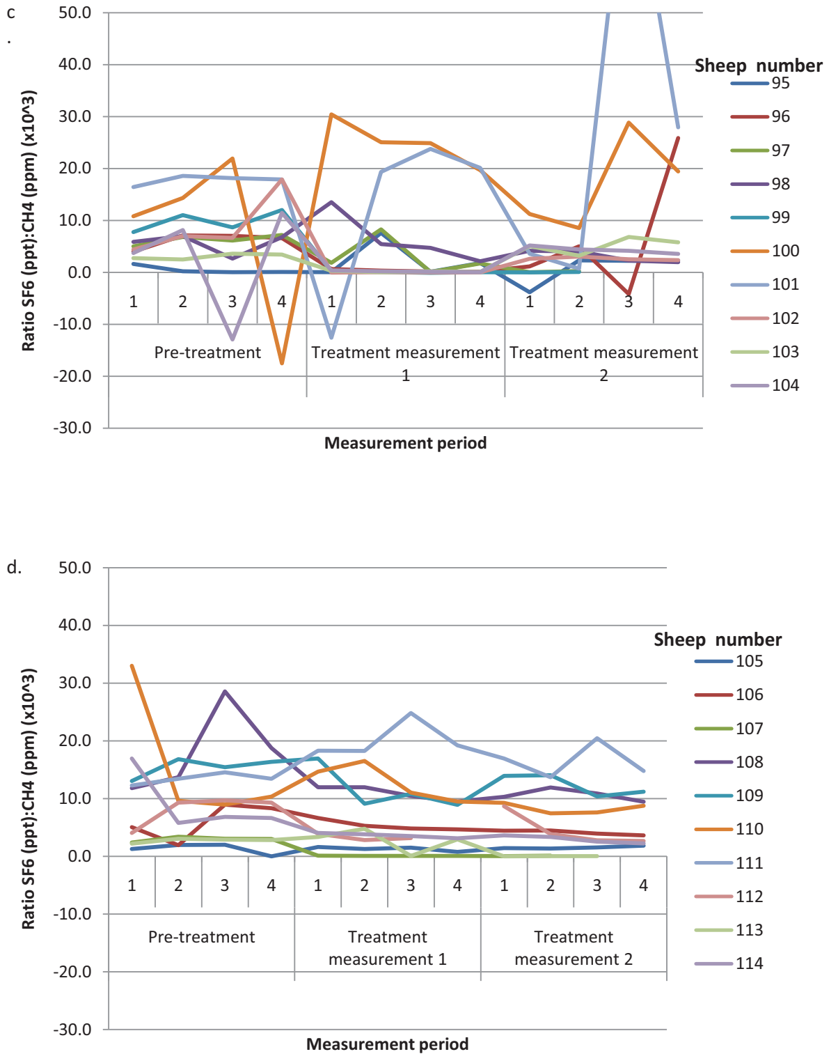
Figure 4.1c.d: Ratio of concentration of sulphur hexafluoride (SF 6 ) and methane (CH 4 ) gases in the breath samples of individual sheep within each measurement period, after correction for ambient concentrations of SF 6 and CH 4 . Each graph shows a sub-group (n = 10) of animals that is not related to treatments or diets fed.
