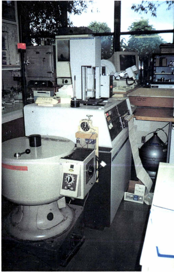
Plate 2.2.4.1 X-ray diffraction machine (XRD) (centre), the orange light on the left hand side indicates that the process is active. Diffraction patterns are being printed on the thermograph paper exiting the unit on the right hand side of the photo. In front of the XRD is the centrifuge (lower left hand corner) that is used in particle size separation (photo: M. A. D'Ath ).
