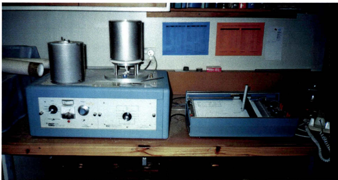
Plate 2.2.6.1 DTA machine. The main unit is shown on the left, with one furnace in place as active and a spare furnace is upside down cooling. On the right hand side the attached printer is producing a DTA pattern (photo: M. A. D'Ath ).
