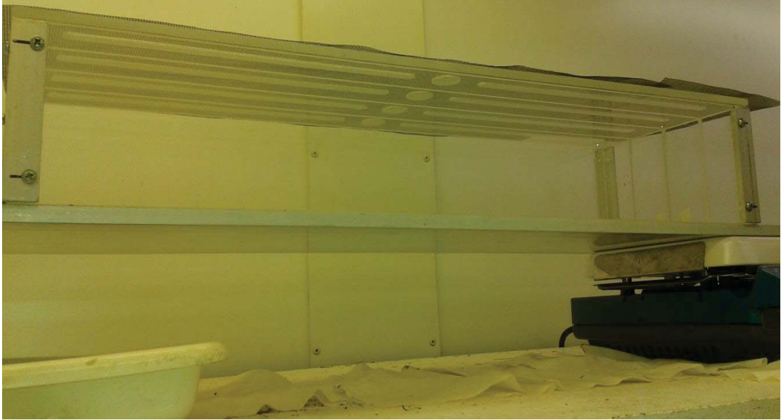
Figure 2.1: Gradient apparatus used for preferred temperature experiment on Phaulacridium marginale individuals.
