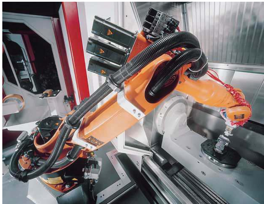
Figure 2.1: An articulated robot moving a work piece between stations (Photo courtesy of Berthold Hermle AG)
