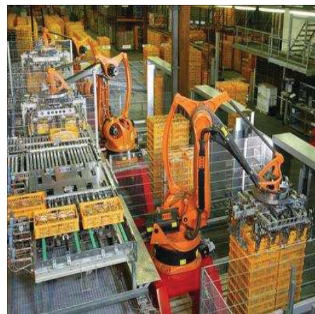
Figure 2.3: An articulated or Z type robot for palletising within a bakery. (Image curtsey of Kuka[80])
