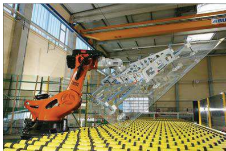
Figure 2.2: An articulated robot handling a glass panel (Image courtesy of Kuka[80])
