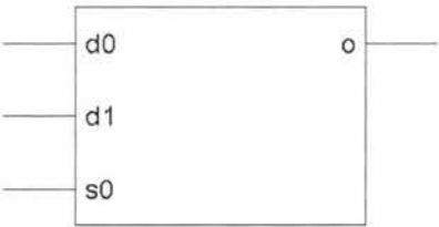
Figure 4.9 Resulting top level RTL symbol for the synthesized 1-bit 2-to-1 multiplexer.
