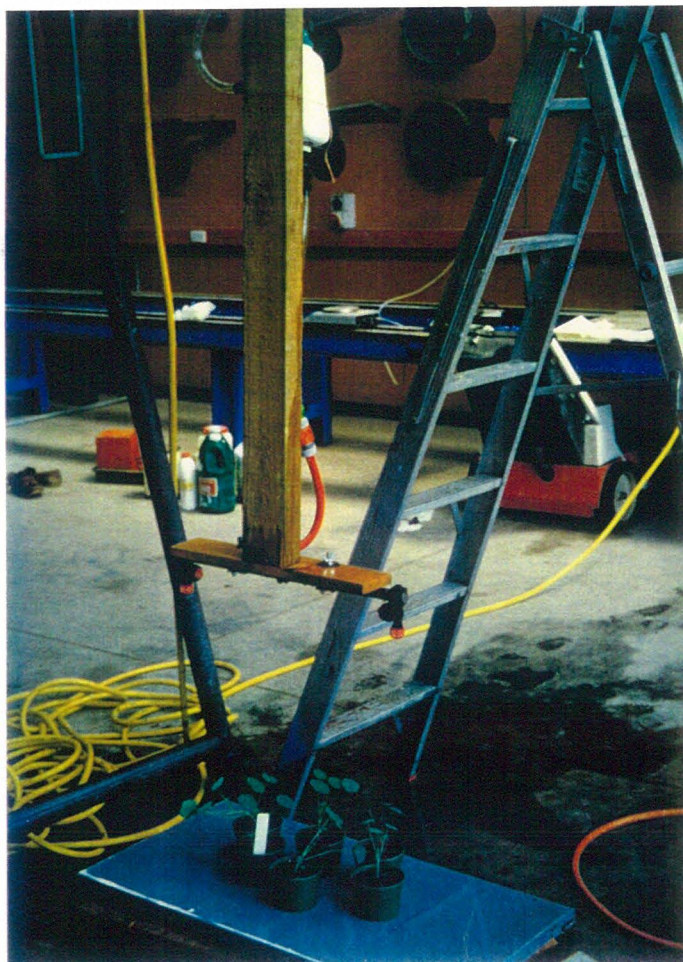
Plate 4.1 Pendulum sprayer design for pots spray.
