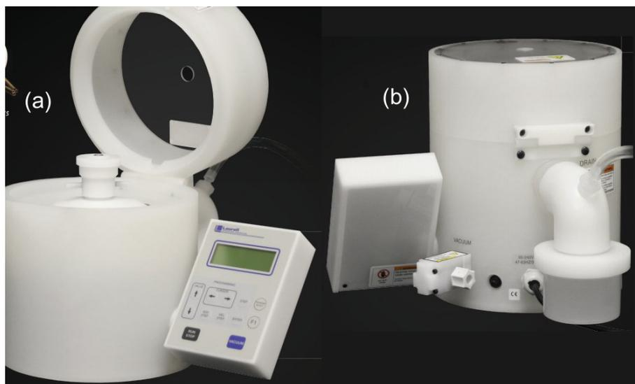
**Figure 3.1** – A WS-400E-6NPP-LITE spin processor by Laurell Technologies Corporation. (a) Front view and (b) Rear-view of the instrument.
