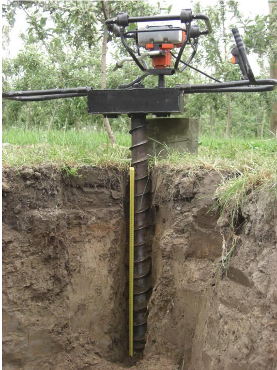
Figure A 3.1.1: Photo of the drill soil corer put 1 metre depth in the soil. The block of wood between the soil surface and the black rectangular gear box was used as a measure to stop the drilling.
