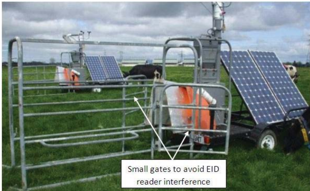
Photograph 4.1: The Sled chute attached to Greenfeed unit with two gates placed near the feeding station and reader to avoid the ear tags of cows outside the unit being identified by the electronic identification reader.
