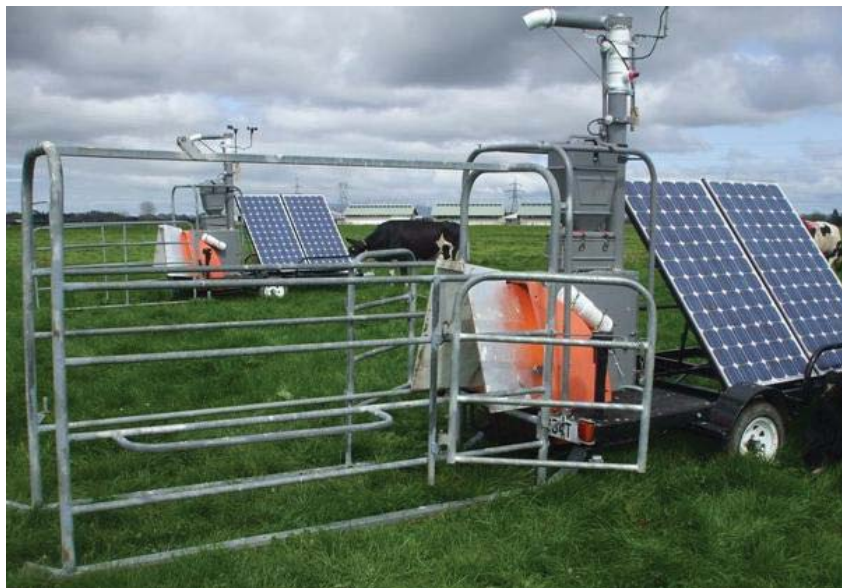
Photograph 2.3: A Greenfeed unit for use by pasture-grazing cows.
