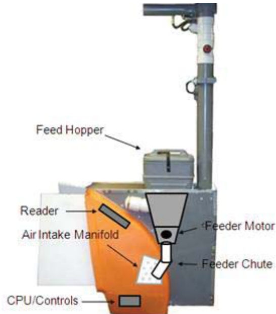
Figure 2.8: Components of the Greenfeed system design. From C-Lock Inc. (unpublished)
