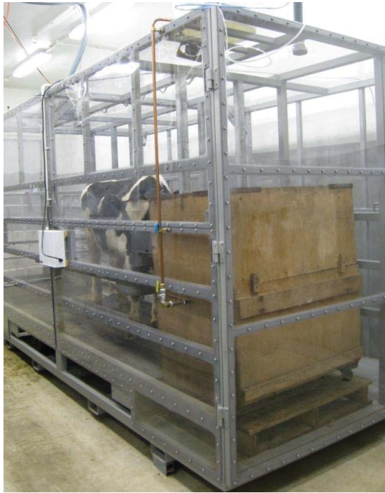
Photograph 2.1: A cow within a respiration chamber at the New Zealand Ruminant Methane Measurement Centre, AgResearch Grasslands, Palmerston North. From Hammond (pers. comm.).
