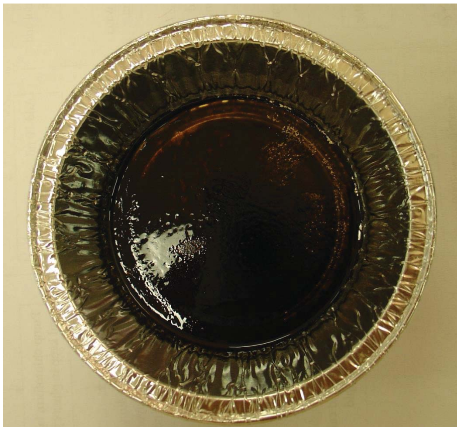
Figure 3.14. The crude oil from microalgal biomass in a preweighed aluminium dish.
