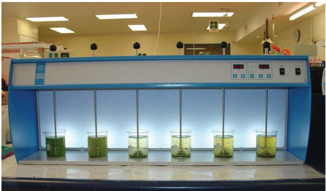
Figure 3.16. A jar test unit for flocculation experiments. The microalgal broth samples (200 mL) in the six beakers were identical but had been dosed with different quantities of the flocculant.
