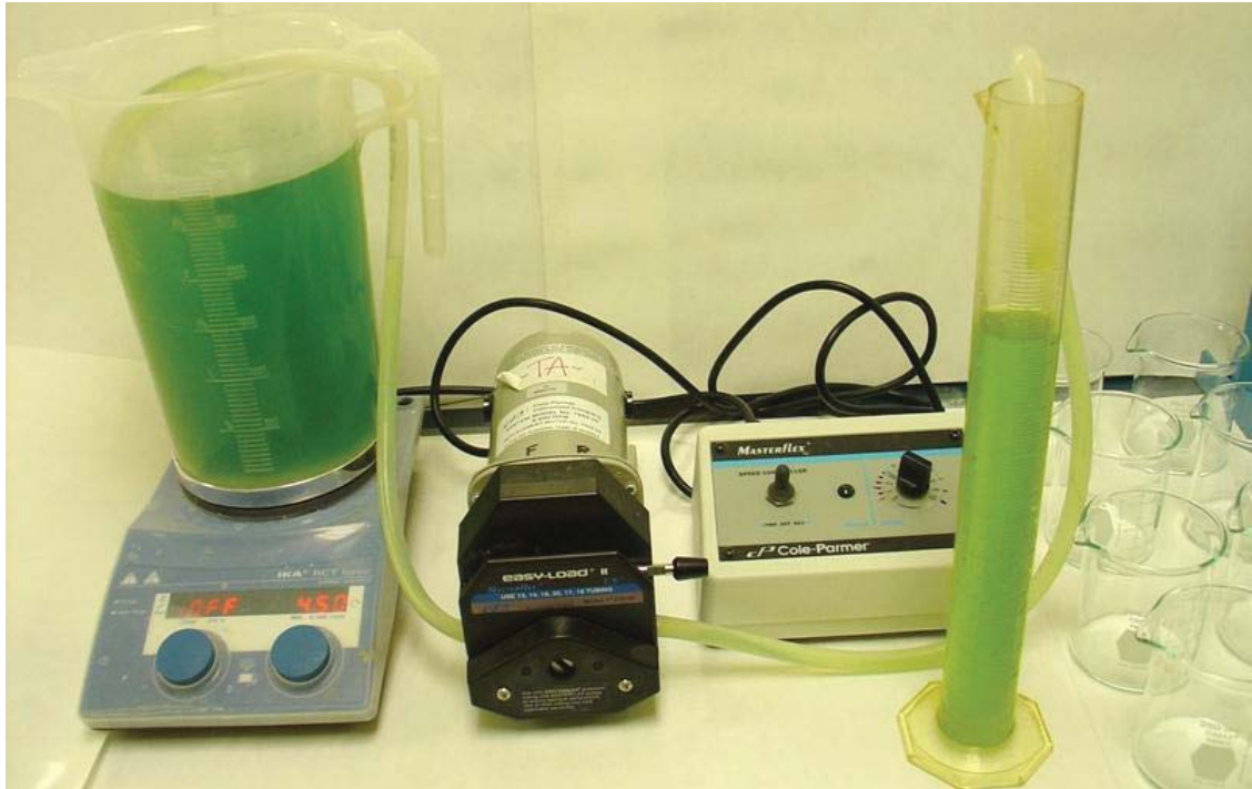
Figure 3.15. Preparation and dispensing microalgal broth in 250 mL beakers for batch flocculation experiments.
