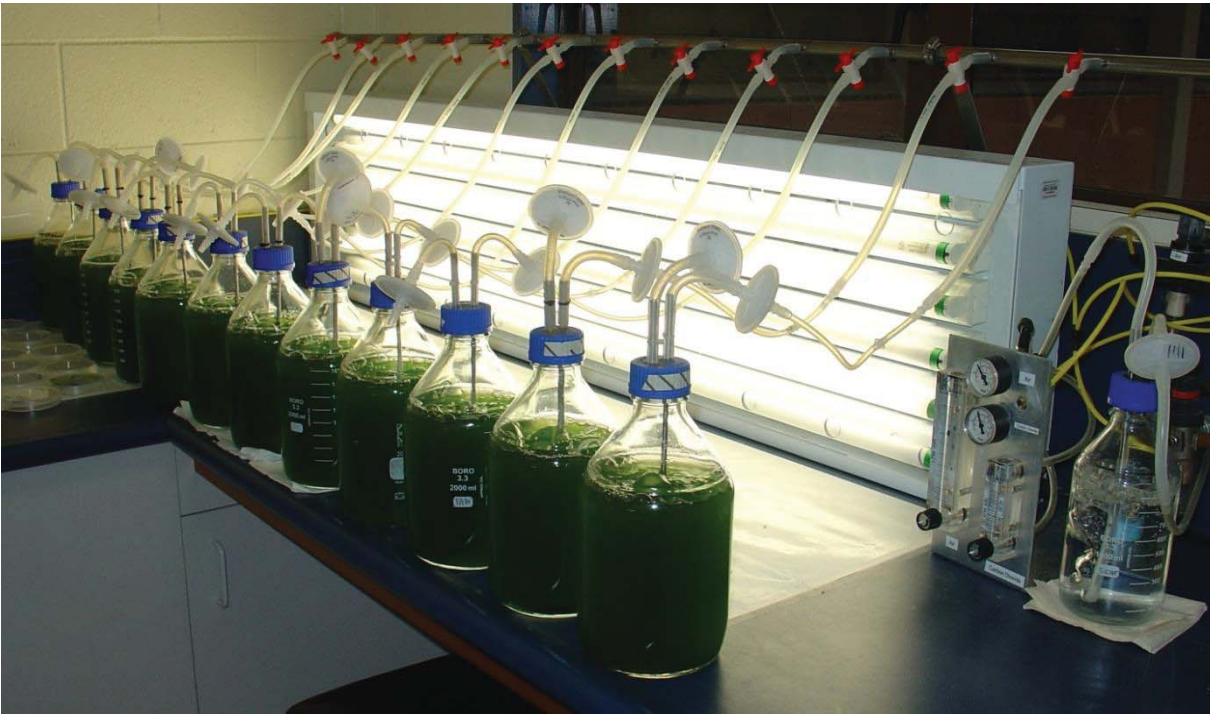
Figure 3.2. Batch culture of microalgae in 2 L Duran bottles. The bottles are being bubbled with a prehumidified mixture of air and carbon dioxide.
