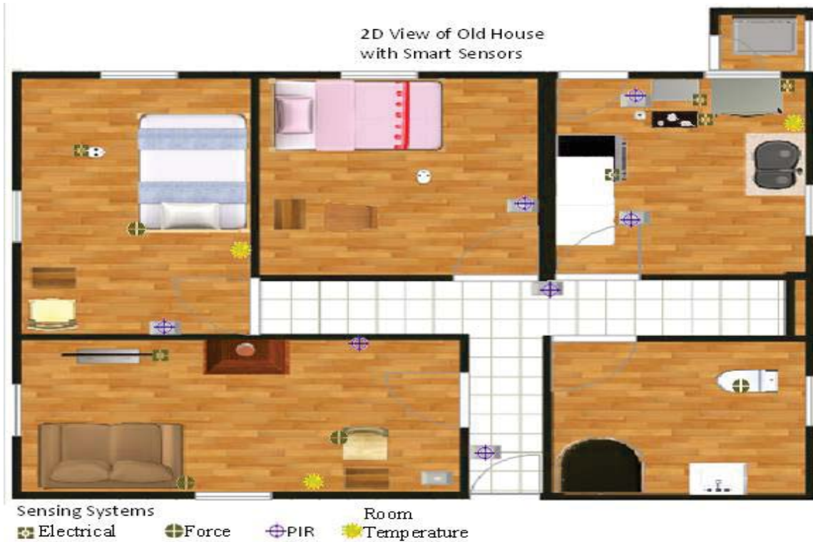
Figure 3-12 2D-View of the house and the placement of different Sensing Systems
