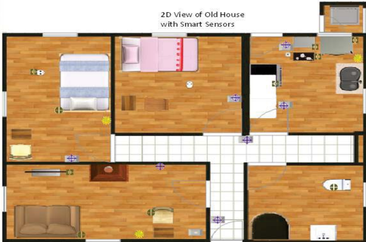
Figure 7-3 Placement of the PIR sensing systems inside the home
