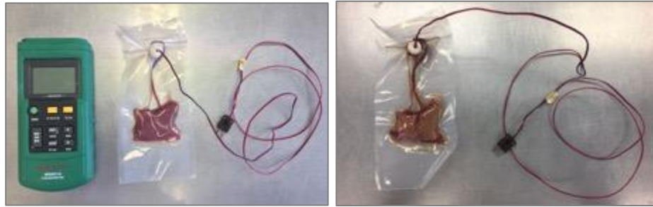
Supplementary figure 1.1 Thermocouple and temperature meter used for monitoring meat temperature during sous vide cooking.
